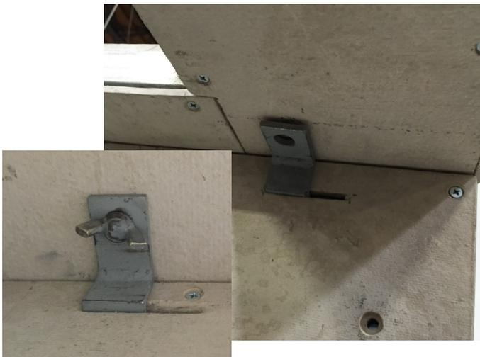
Secure the top panel (GT) to the rear panel (GR) in 4 places using small angle brackets with Medium Large wing
