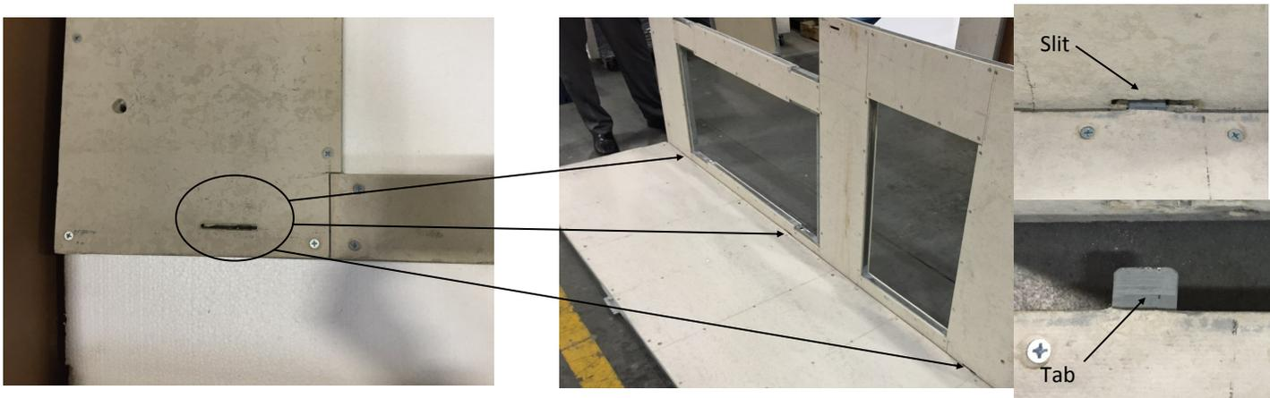
Assemble side (*GS*) and front panels (*GF*) together using **4** medium wing bolts to secure to the panels . Depending on your orientation (left or right side) you will attach the side panel (*GS*) on the grill island on the end that will be exposed.
